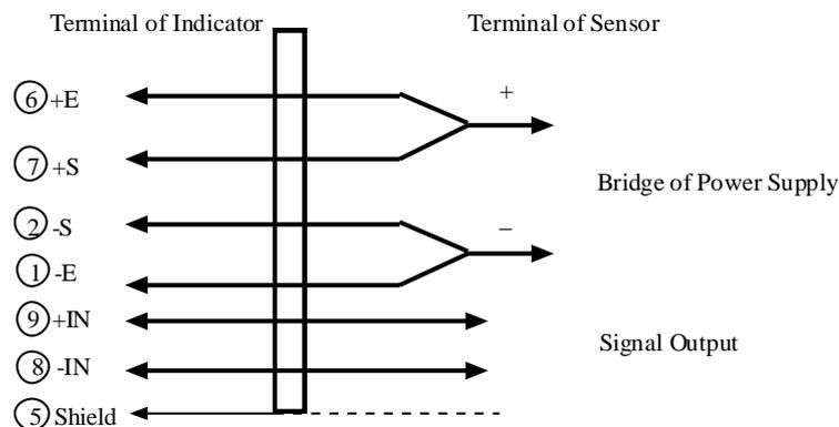
Connection of the load cell
