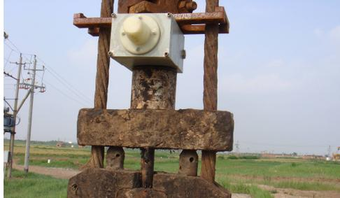
Petro pump have two main behaviour, rise and down process,both process effected on the load cell with different direction, the smallest stress probably in about 3 ~ 5t, the largest in 9 ~ 12t or so (different wells with different value). Waveform curve as shown below:
