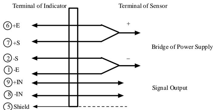
Connection of the load cell
