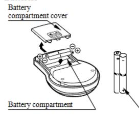
Remove the battery compartment cover and insert four batteries(R6P/LR6 /AAAsize) into the battery compartment, taking extreme care that the polarities plus and minus is observed.
