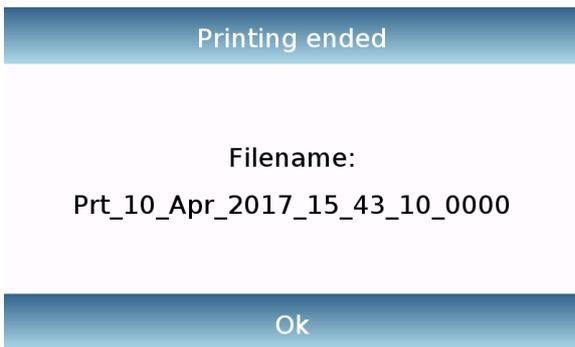
➤ **File on Usb-Key:** command print, touching the "Print" button will print to file. In order to use this mode, you will need a USB stick to save the files. (You can use a dedicated USB stick for that purpose only). With the "File on Usb\_Key enabled" mode before executing the print command, verify that the save USB stick is inserted in the USB port on the left side of the device. While saving the file on the screen, you can scroll through the information that will be saved in the file.
