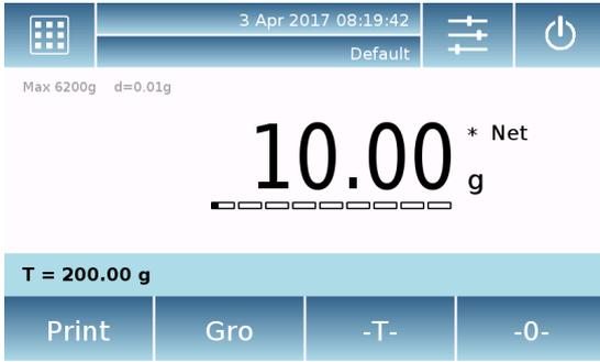
Place the material to weight on the balance and wait for the stability symbol to light up before detecting the value.
