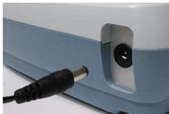
**Insert** the supplied power supply unit jack into the connector on the back of the device.
