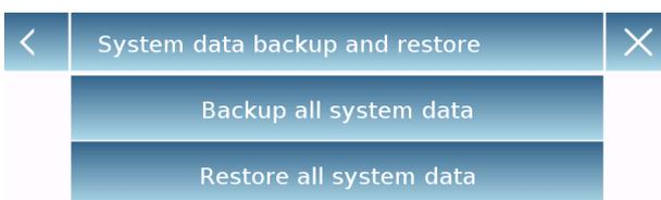
You can back up the system completely or restore data and configuration previously saved on a USB stick.
