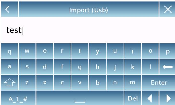
If the USB stick is inserted correctly, after confirmation, the alphanumeric keypad will automatically be displayed for entering the name of the backup you want to restore.
